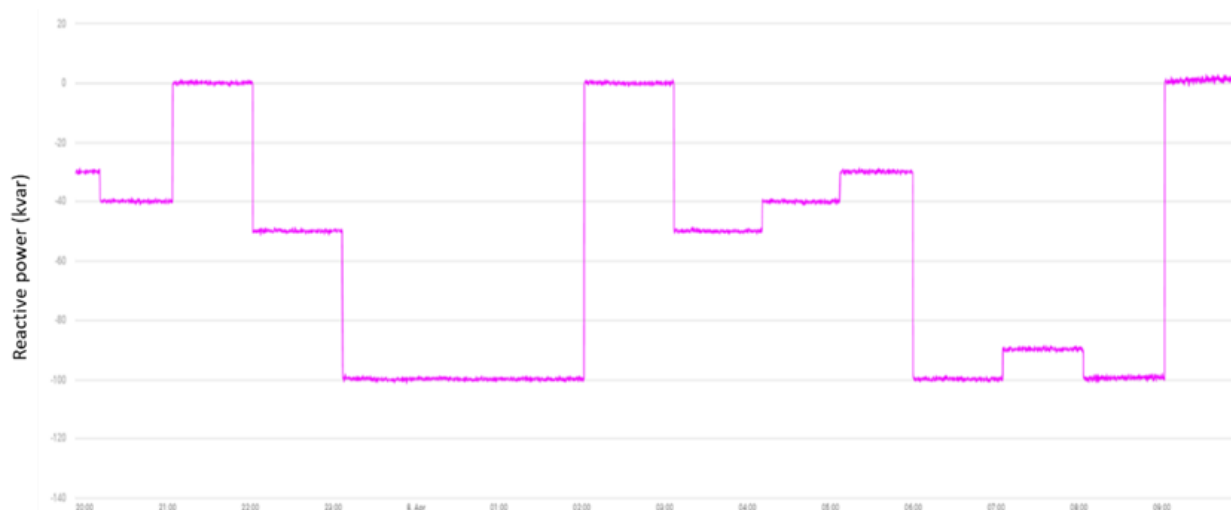
FIGURE 42. REACTIVE POWER COMPENSATION TESTS ACCORDING TO A CALENDAR-BASED SCHEDULE WITH ONE OF THE INVERTERS OF KIVIKKO PV PLANT, APRIL 2020. MINUS: REACTIVE POWER CONSUMPTION. PLUS: REACTIVE POWER PRODUCTION.
