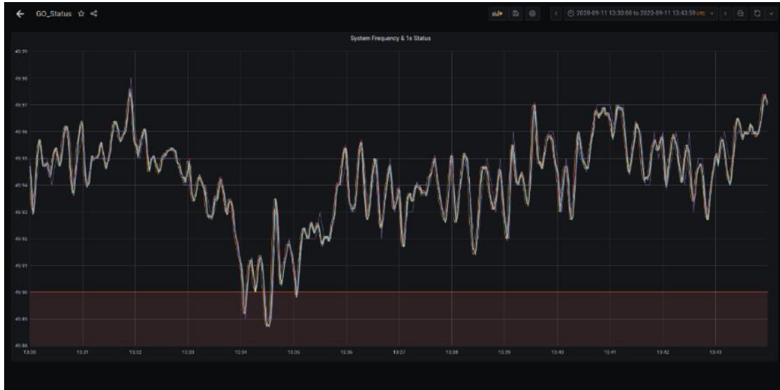
FIG. 5 REFINED FREQUENCY MEASUREMENT FROM BATTERIES VS SYSTEM FREQUENCY FROM EIRGRID
