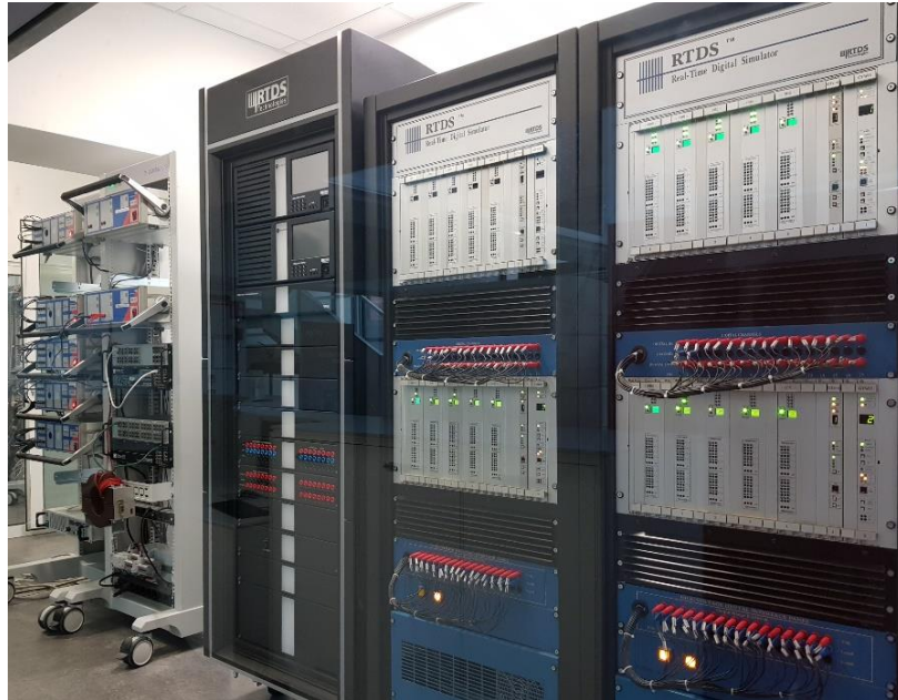
FIGURE 3-6 - RTDS RACKS IN LAB FACILITIES CONNECTED TO VOLTAGE AND CURRENT AMPLIFIERS.
